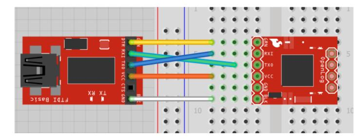
It's easiest to use a breadboard to make the connection from an FTDI to an OpenLog.
